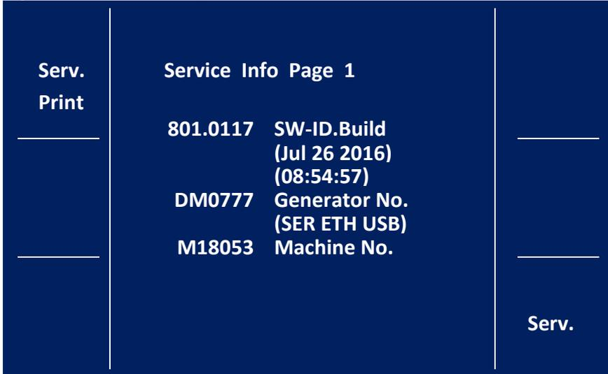
If you press „Serv.“-button again, you'll see cooling water flow (sensor 0), generator temperature (IGBT) and actual machine state. The rows 'Water flow 1' and 'Op.' are not used in MC16. The button 'Serv. (Service) Print' is without function.
