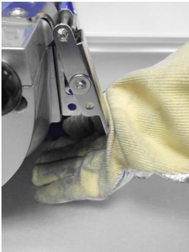
Close the lock with the ball of hand. Hold the hand open and use a glove.
